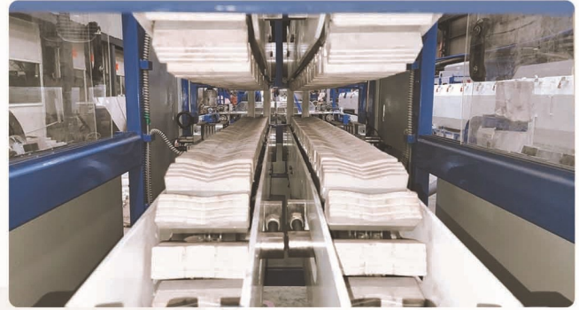
SIDE VIEW OF DUAL HDPE PIPE HAUL-OFF
