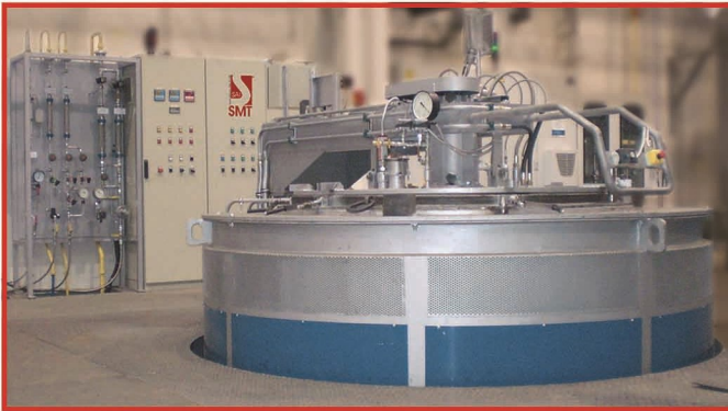
GAS NITRIDING FURNACE
